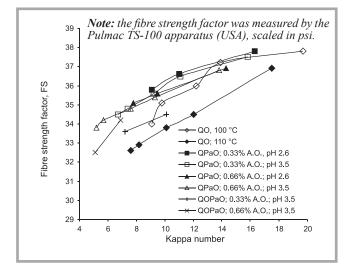
Figure 5. Relationship between zero-span fibre strength factor and kappa number of oxygen-delignified pine kraft kappa number 31.5 pulp in different variants of the process (after beating the pulp in a Jokro mill to freeness 20°SR, beating time 12 min.); (Standard deviation of FS-factor was 1.1).
