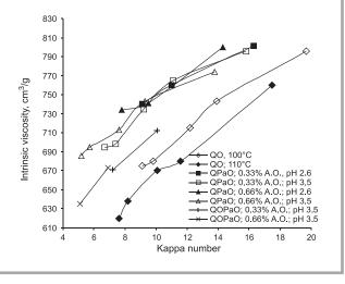
**Figure 4.** Relationship between kappa number and intrinsic viscosity of oxygen-delignified pine kraft kappa number 31.5 pulp in different variants of the process. (Standard deviation of viscosity was  $8 \text{ cm}^{3/g}$ ).
