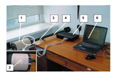
View of the TEXTILPRESS measuring stand during measuring; 1—textile compression band, 2—measuring matrix placed under the band, 3—cylinder, 4—cylinder holder, 5—data acquisition system, 6—computer.
