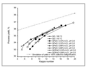
**Figure 2.** Yield-to-kappa number relationship in different variants of oxygen delignification of pine kraft pulp, kappa number 31.5. (Standard deviation of yield amounted to 0.14%).
