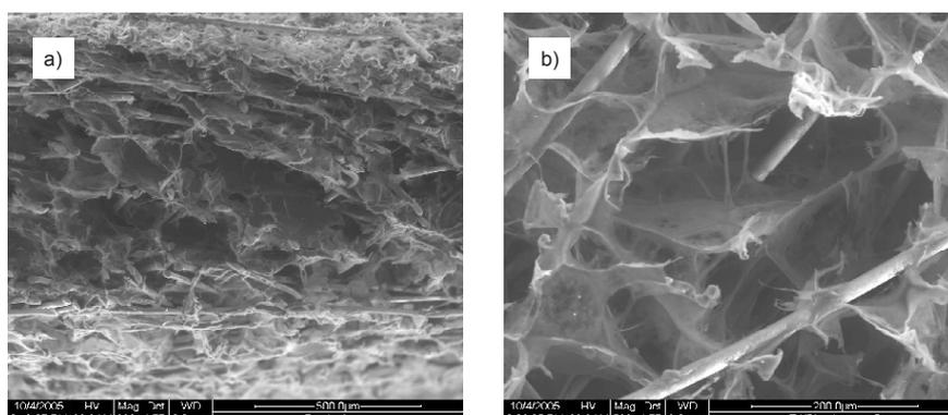
**Figure 3.** Chitosan sponge with an addition of PP fibres including Irguard B 7000; a) cross-section, magnitude 200×, b) sponge surface, magnitude 500×.
