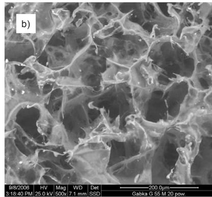
**Figure 4.** Surface of M20-5.0 chitosan sponges; a) magnification 200 $\times$ , b) magnification 500 $\times$ .
