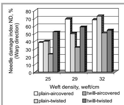
**Figure 4.** The variation of needle damage index in the warp direction, according to weft density.
