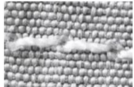
**Figure 5.** Appearance of the lockstitch on fabric BPA3PE.
