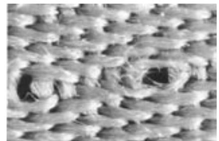
**Figure 8.** Appearance of the needle perforation in the warp direction of fabric DTA1PE.
