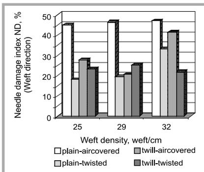
**Figure 3.** The variation of needle damage index in the weft direction, according to weft density.
