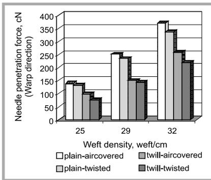
**Figure 1.** The variation of needle penetration forces in the warp direction, according to the weft density.
