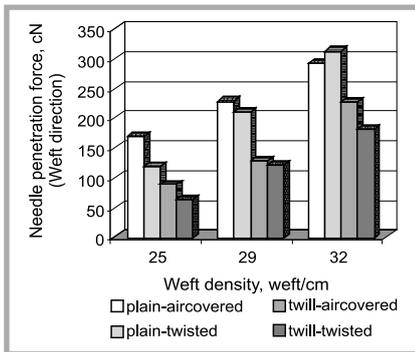
**Figure 2.** The variation of needle penetration forces in the weft direction, according to the weft density.
