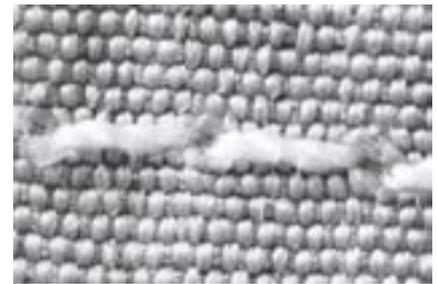
**Figure 6.** Appearance of the lockstitch on fabric BTA1PE.
