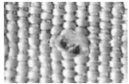
**Figure 7.** Appearance of the needle perforation in the warp direction of fabric BTA3PE.
