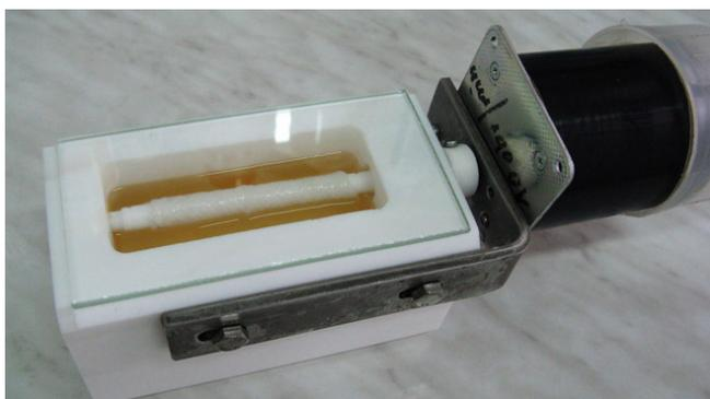
**Figure 3.** Dynamic culture in a reactor with a rotating PTFE shaft and the polyester vein reinforcement applied - BR-1 (Tricomed SA).
