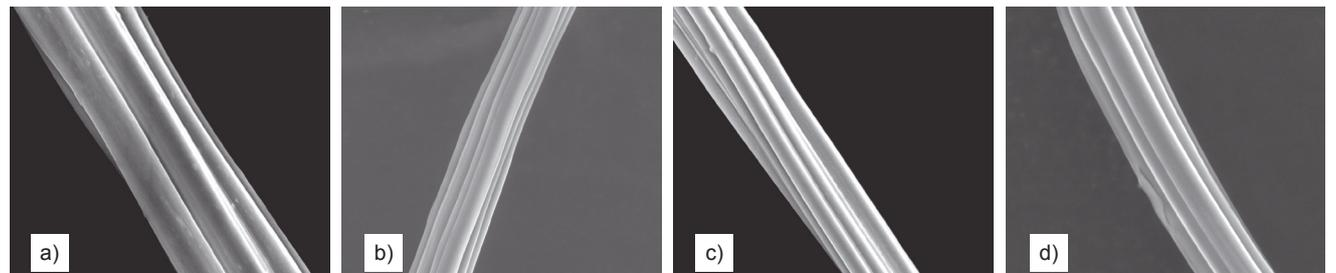
**Figure 5.** Longitudinal view of the fibres investigated: a) viscose fibre, b) “bamboo fibre” from yarn, c) “bamboo fibre” from knitted fabric, d) “bamboo fibre” from woven fabric (weft), (magnification 6000×).
