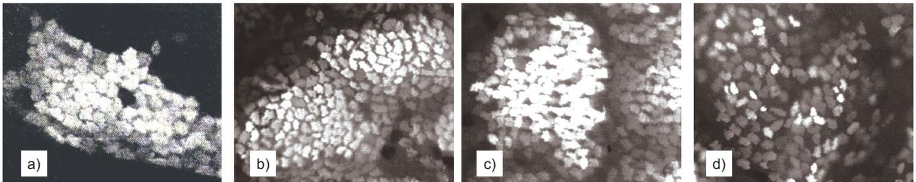
**Figure 4.** a) Cross-section of viscose fibres [17], b) Cross-section of “bamboo fibres” from yarn, c) Cross-section of “bamboo fibres” from knitted fabric, d) Cross-section of “bamboo fibres” from woven fabric (magnification 200×).
