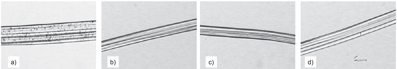
**Figure 3.** Longitudinal view of the fibres: investigated a) viscose fibre, b) “bamboo fibre” from yarn, c) “bamboo fibre” from knitted fabric, d) “bamboo fibre” from woven fabric (weft), (magnification 200×).
