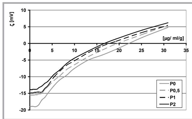
Figure 4. Zeta potential ( $\zeta$ ) of the cotton fabrics vs. ionic surfactant addition (N-CPC) in 0.001 M KCl at pH 10.
