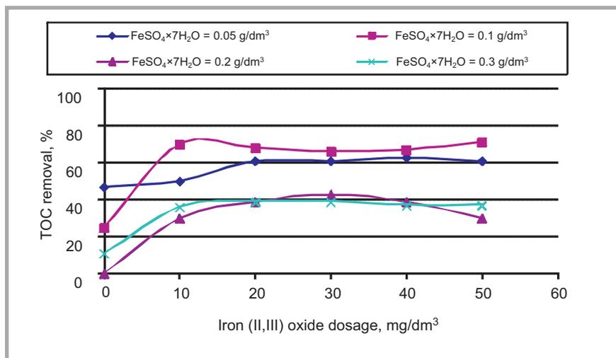
**Figure 5.** Effect of ferrous sulfate and iron oxide nanopowder on TOC removal in C.I. Direct Yellow 86 dye solution in the nanoFenton process. Hydrogen peroxide dosage – 2 cm<sup>3</sup>/dm<sup>3</sup>, initial TOC = 27.9 mg/dm<sup>3</sup>, pH 3.5.
