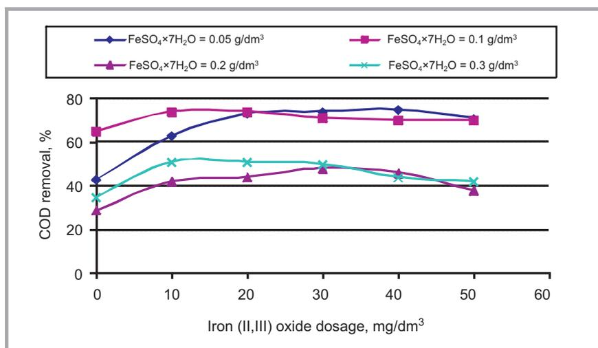
**Figure 4.** Effect of ferrous sulfate and iron oxide nanopowder on COD removal in C.I. Direct Yellow 86 dye solution in the nanoFenton process. Hydrogen peroxide dosage – 2 cm<sup>3</sup>/dm<sup>3</sup>, initial COD = 84 mg O<sub>2</sub>/dm<sup>3</sup>, pH 3.5.
