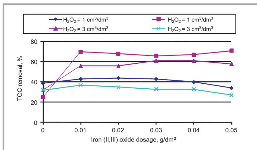
**Figure 7.** Effect of iron oxide nanopowder dosages on TOC removal in C.I. Direct Yellow 86 dye solution in the nanoFenton process at different quantities of hydrogen peroxide added to the system. Ferrous sulfate dosage – 0.1 g/dm<sup>3</sup>, initial TOC = 27.9 mg/dm<sup>3</sup>, pH 3.5.
