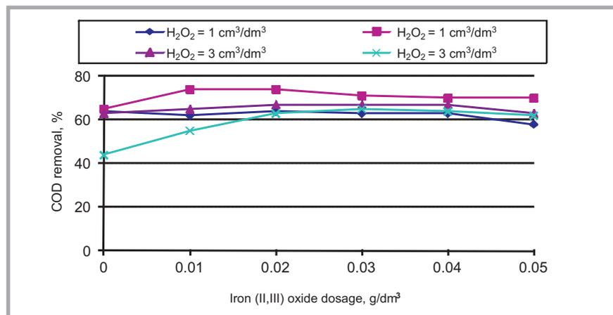
**Figure 6.** Effect of iron oxide nanopowder dosages on COD removal in C.I. Direct Yellow 86 dye solution in the nanoFenton process at different dosages of hydrogen peroxide introduced to the system. Ferrous sulfate dosage – 0.1 g/dm<sup>3</sup>, initial COD = 84 mg O<sub>2</sub>/dm<sup>3</sup>, pH 3.5.
