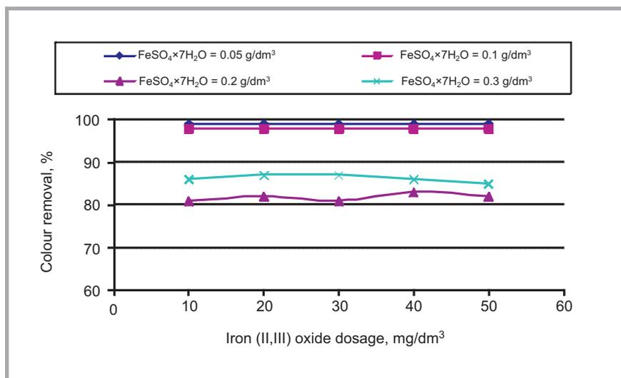
**Figure 3.** Effect of ferrous sulfate and iron oxide nanopowder on colour removal in C.I. Direct Yellow 86 dye solution in the nanoFenton process. Hydrogen peroxide dosage – 1 cm<sup>3</sup>/dm<sup>3</sup>, initial absorbance – 4.45 (wavelength 364 nm), pH 3.5.
