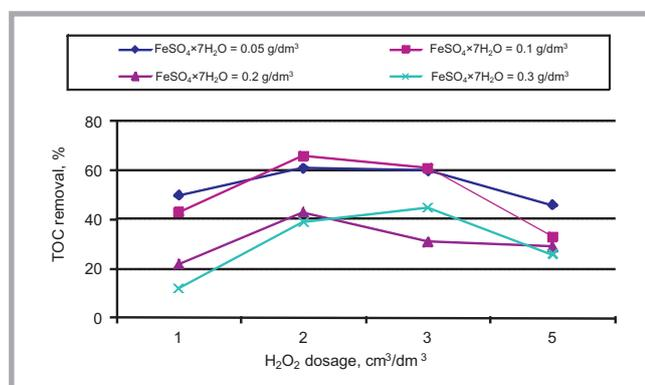
**Figure 10.** Effect of hydrogen peroxide dosages on TOC removal in C.I. Direct Yellow 86 dye solution in the nanoFenton process at different dosages of ferrous sulfate. Dosage of iron oxide nanopowder – 0.03 g/dm<sup>3</sup>, initial TOC = 27.9 mg/dm<sup>3</sup>, pH 3.5.
