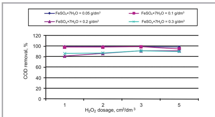
**Figure 8.** Effect of hydrogen peroxide dosage on colour removal in C.I. Direct Yellow 86 dye solution in the nanoFenton process at different ferrous sulfate dosages. Dosage of iron oxide nanopowder – 0,03 g/dm<sup>3</sup>, initial absorbance – 4.45 (wavelength 364 nm), pH 3.5.
