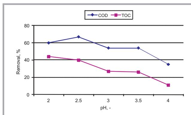
**Figure 11.** Effect of the pH on COD and TOC removal in C.I. Direct Yellow 86 dye solution in the nanoFenton process. Dosages: ferrous sulfate – 0.3 g/dm<sup>3</sup>, iron oxide nanopowder – 0.03 g/dm<sup>3</sup>, hydrogen peroxide – 3 cm<sup>3</sup>/dm<sup>3</sup>, initial COD = 84 mg O<sub>2</sub>/dm<sup>3</sup>, TOC = 27.9 mg/dm<sup>3</sup>.
