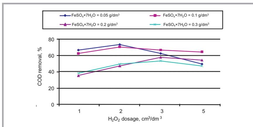
**Figure 9.** Effect of hydrogen peroxide dosage on COD removal in C.I. Direct Yellow 86 dye solution in the nanoFenton process at different ferrous sulfate dosages. Dosage of iron oxide nanopowder – 0.03 g/dm<sup>3</sup>, initial COD = 84 mg O<sub>2</sub>/dm<sup>3</sup>, pH 3.5.
