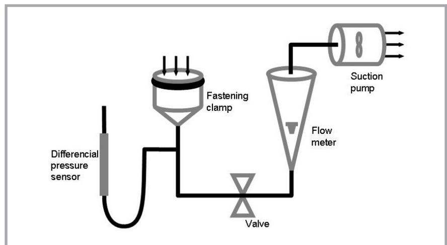
**Figure 1.** General diagram of the device for air permeability measurement (with a suction-pump) [5].
