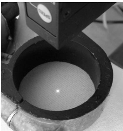
Figure 6. Bulge measurement using laser.
