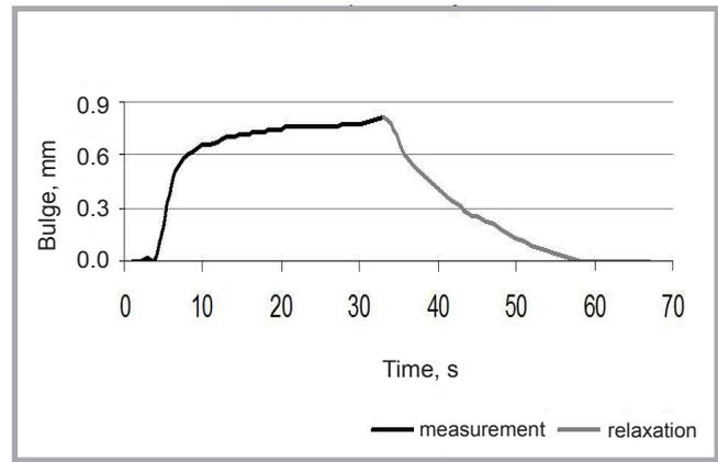
Figure 9. Bulge of the sample and subsequent relaxation, time-dependent.
