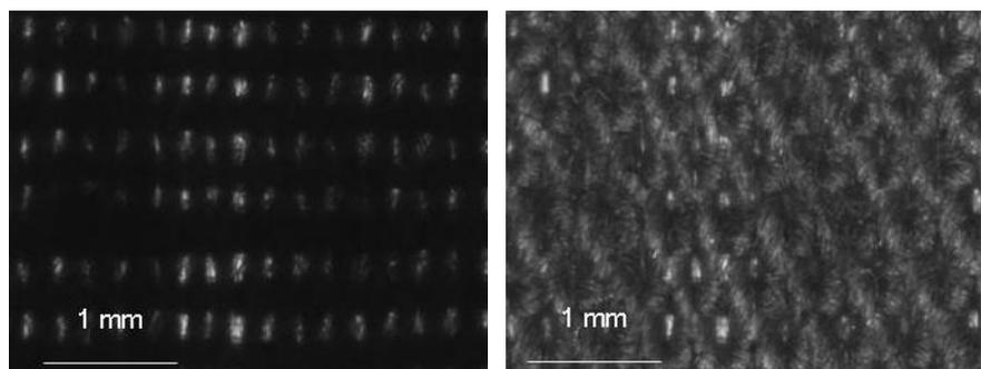
Figure 5. Photograph of a woven textile without illumination from above (left) and with illumination from above (right).
