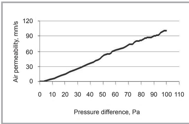
Figure 8. Example of data with a pressure difference measurement step.
