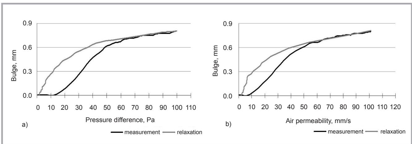
Figure 10. Example of graphs depicting the bulge of the sample depending on increasing pressure (a) and air permeability (b).
