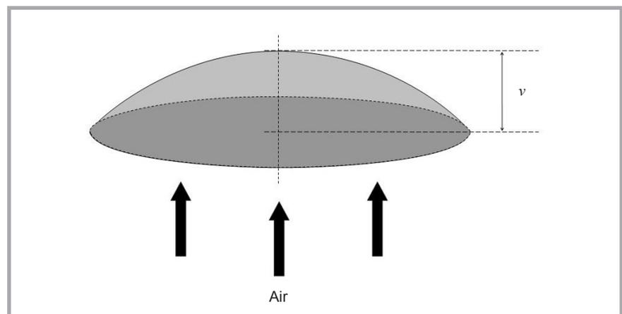
Figure 7. Schematic image of a sample bulge of magnitude  $v$ .
