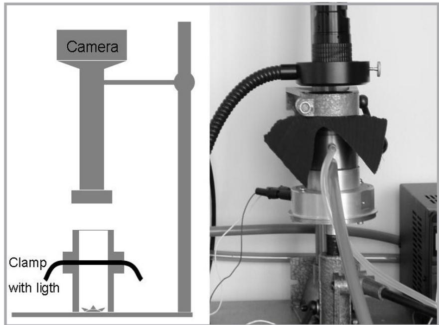
Figure 4. Fastening clamp adjusted to enable observation of the structure of the textile.
