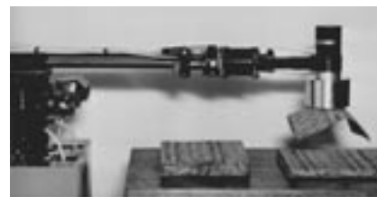
Figure 1. Robotized pick up-device for textile pieces.
